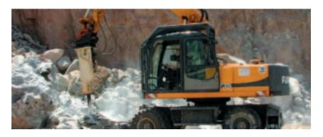
driven by the machine's on-board hydraulic system. Extra drives, auxiliary power or control valves are all redundant.
