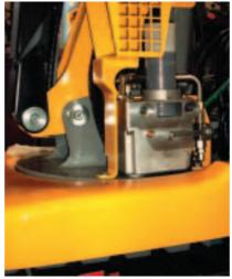
The HTL 101 mounts directly on the accessory, minimizing tubing and drastically reducing installation costs. An integrated over-pressure valve and a selection of three possible lubricant outlet locations makes it easy to find the optimum installation position.
